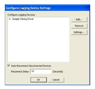
This screen displays all of the currently installed logging devices. It is the place where you can add, remove, and reconfigure the devices that WinLog will communicate with. In some instances, the logging device can be a simple driver, and not have any hardware (such as the WinLog Performance Monitor), in other cases, hardware and software are required to make the device work. Up to 64 devices can be installed simultaneously in WinLog.
